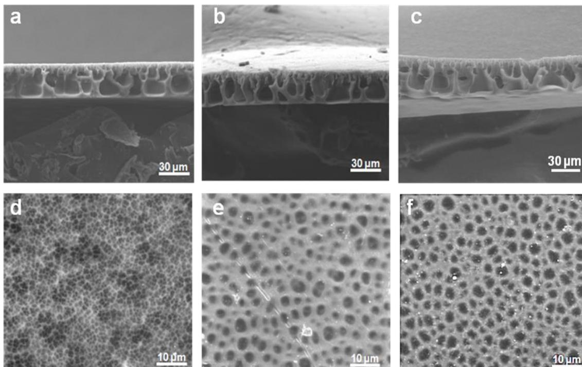
Figure 2: Cross-section (a: Phase Inversion, b: Phase Inversion + Nanosilica, c: Phase Inversion + Nano Calcium Carbonate) and Surface SEM Images (d: Phase Inversion, e: Phase Inversion + Nanosilica, f: Phase Inversion + Nano Calcium Carbonate) of Porous Polybenzimidazole
